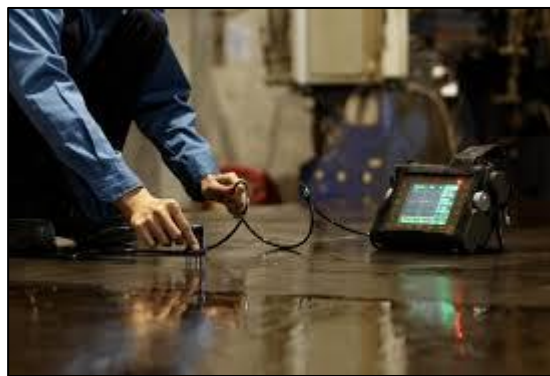
(Figure 1 Ultrasonic Testing - https://nationalndt.co.za/services/ultrasonic-testing/ )
