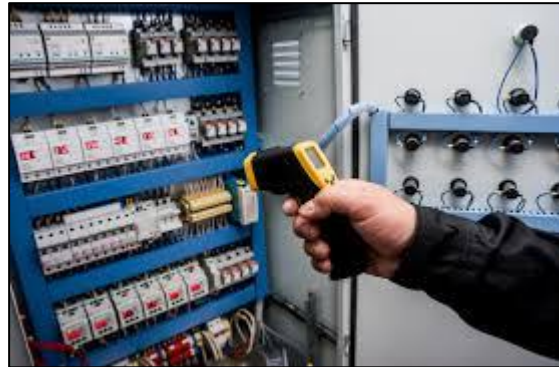
(Figure 4 Thermographic Testing - https://ocean-me.com/the-benefits-of-infrared-thermography-testing/ )
