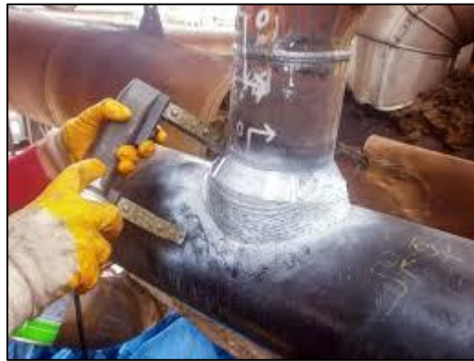
(Figure 2 Inspection of magnetic particles - https://www.flyability.com/blog/magnetic-particle-inspection )
